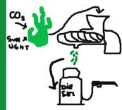
After initial growth, algae is deprived of nutrients (carbon dioxide, sunlight and others) to produce a greater oil yield. Then, by extraction, the press produces 75% of the oil from the plant. Ready oil can be used directly in diesel engines. Algae is one of the fastest growing plants.
