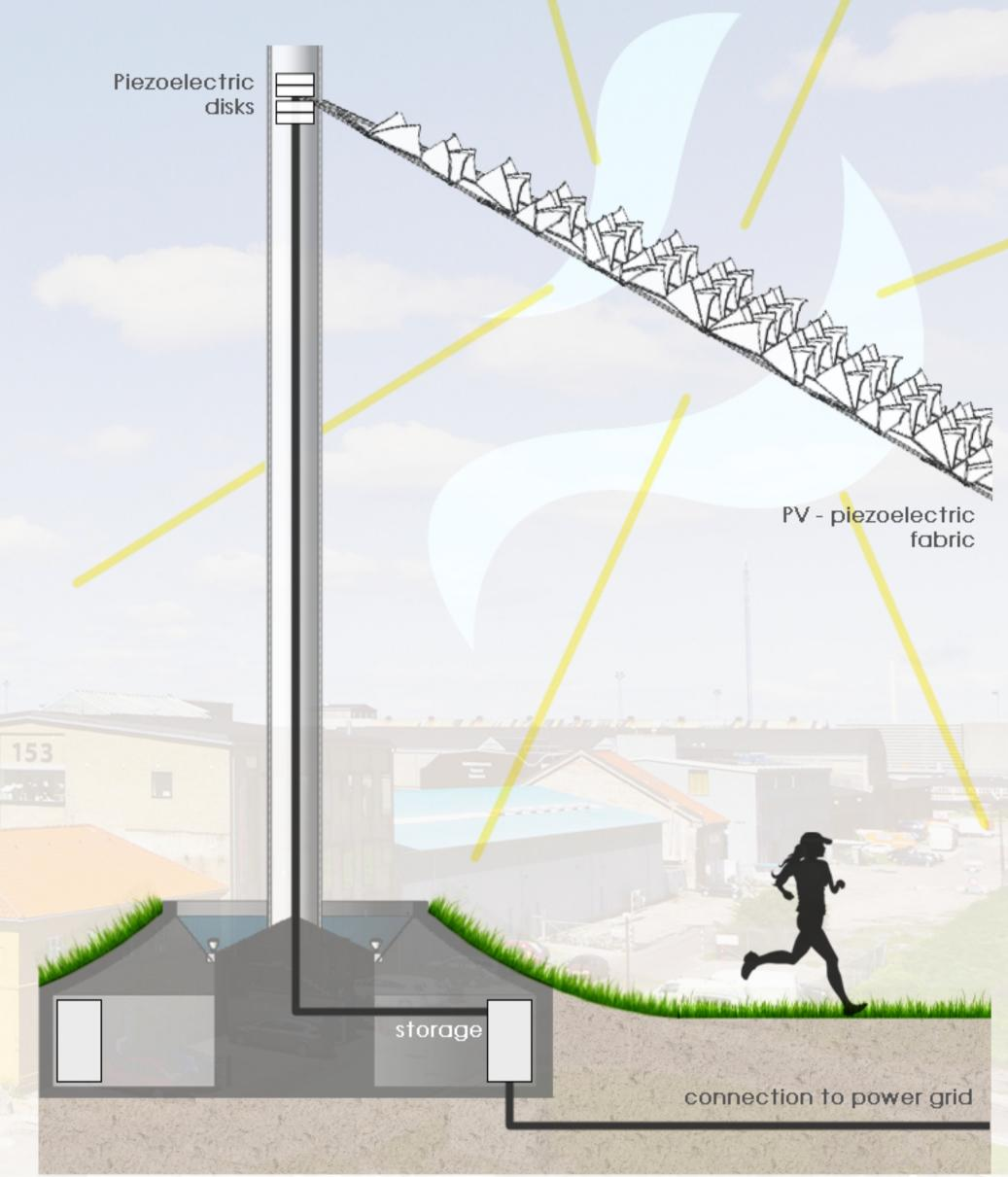
The conceptual salls are technically tensed conductive nets supported on several masts or posts. The generation occurs on pieces of cloth attached to this grid. But the net itself is a regular grid composed of loose electrical conductors inside flexible plastic tubes; being the latter the ones that are truly subjected to the structural tension.
