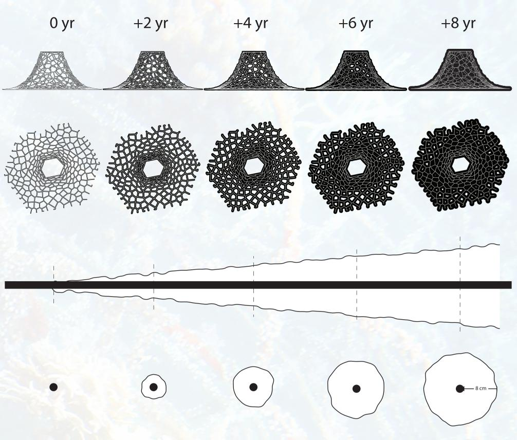
Over time, the lattice form-work begins to solidify, growing at a rate of 1-2 cm per year. In the event of damage, concrete will form more rapidly around exposed areas of metal. As long as the current continues to flow, rust will not form on the sub structure.
