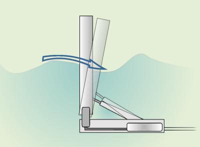
WATER BURSTING INTO THE GRASPER MAKES IT BEND AND PUT THE PUMP IN MOTION.
