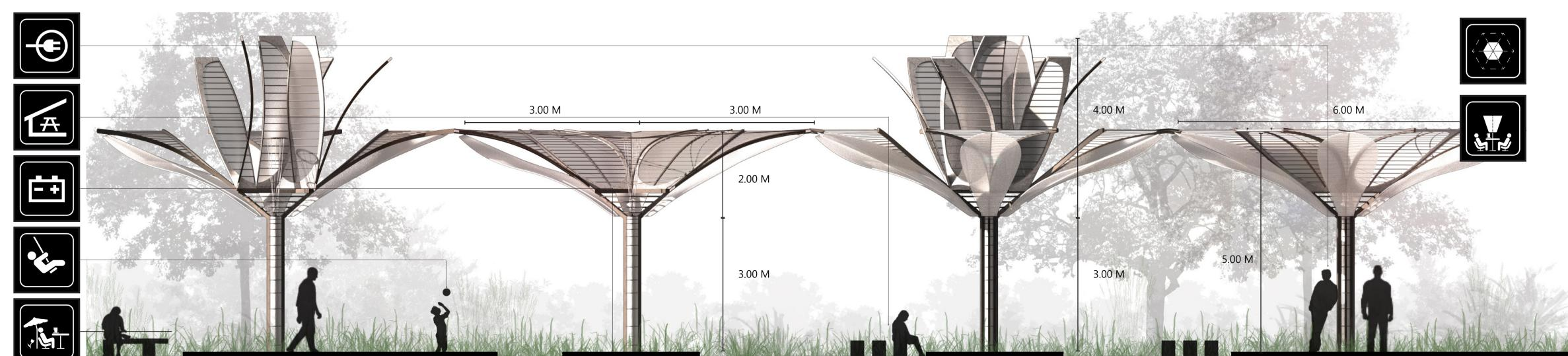
The solar-shades closes like a flower permitting the project exist in two different states. During the day, the retractable arms are open permitting the maximum solar energy harvesting and creating a soft continuity in the space providing a 65 percent of shadowing under and making possible host all kind of temporary activities, concerts, festivals, private events, and exhibitions or public demonstrations.
