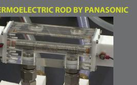
suck 2.5 watts of electricity out of hot water running through a 10 centimeter section of water of 10 °C outside the tube. The power density corresponds to as high as 10 kW with
