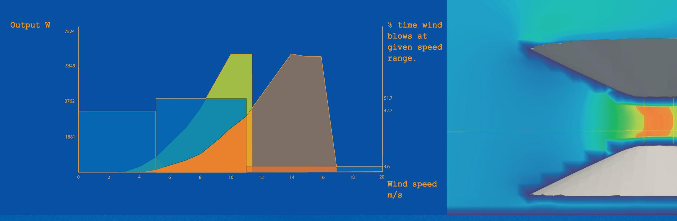
**Power Output** Original power output curve<sup>2</sup> relative to wind speed in orange. New power output curve based on boosting wind speed. The blocks indicate (within speed ranges) the percentage time wind blows. The key to note is that with 'boost' the power output curve overlaps much more of the wind time blocks. <sup>2</sup> http://www.bettergeneration.co.uk/wind-turbine-reviews/qr5-wind-turbine.html accessed on 16/05/2014 at 21:15
