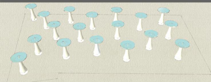
18 Drop columns are designed above the zero level. Each column is 3m diameter and 31m height. External cover of columns is shaped as asymmetrical cone from larger bottom to narrower top. The cover is selected for plant growing surface and providing enough maintenance space to installed pipes on columns.
