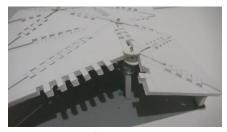
Taking advantage of the site surroundings, we are incorporating wave generating device that collects energy through human movement. The panel would move up and down according to human movement as well as wave movement. There would be an interlocking connection between two panels that allow movement. At each main
