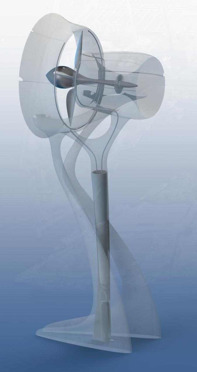
HORN consist of two wind turbines aligned on the same axis, contained within a concrete structure inspired by jet engines and two water reservoirs each powering a different type of turbine.
